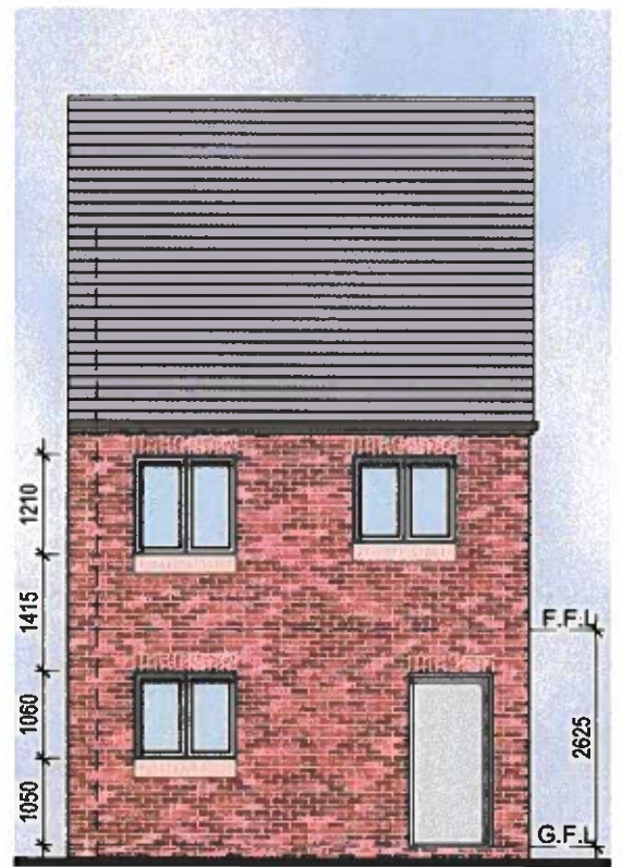
REAR ELEVATION SCALE 1:100
